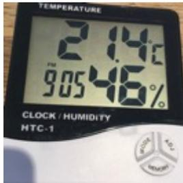
A humidity meter was left. The temperature of the wall was measured and found to be 10.4°C which is below the mould point of 11°C based on the relative humidity of 46%RH and ambient temperature of 21.4°C – use the meter in conjunction with MouldPoint.co.uk.
